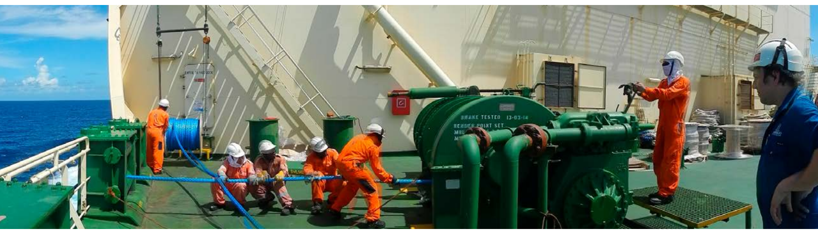
A Samson field service technician inspects each line as it is installed to ensure that it meets Samson's high quality standards.
