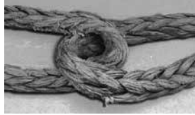
Eye-to-eye splice connection.
