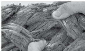
Inspect for internal abrasion
