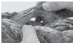
Inspect for pulled strands
