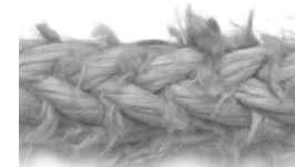
Severely abraded 12-strand rope
