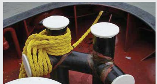
FIGURE 4 Proton-8 with "right" twist.
