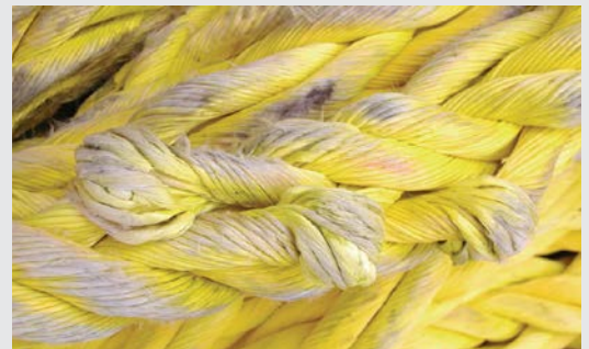
FIGURE 2 Proton-8 with severe strand hockles.
