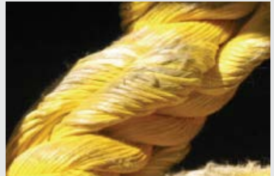
FIGURE 1 Proton-8 with a hockle.
