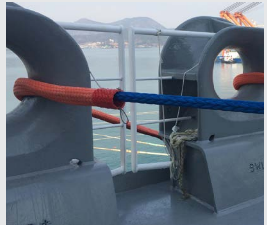
Samson recommends the use of chafe protection for mooring rope contact points.
