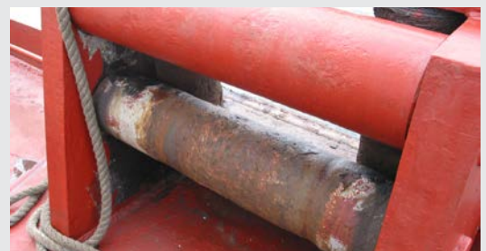
All chocks must be kept free of grooves, pits and/or rust to minimize rope damage potential.
