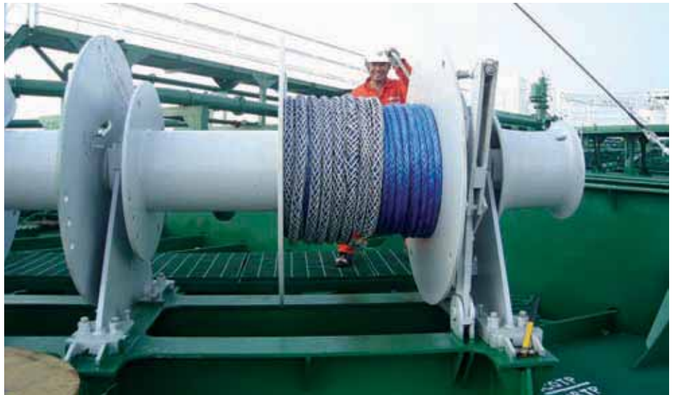
Samson’s AmSteel®-Blue on a test winch.
