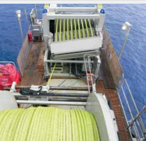
ABOVE: ROV "handling grommets" used by the ROV to maneuver and position the AmSteel®Blue heavy lift grommets.
