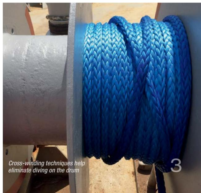
*Cross-winding techniques help eliminate diving on the drum*
