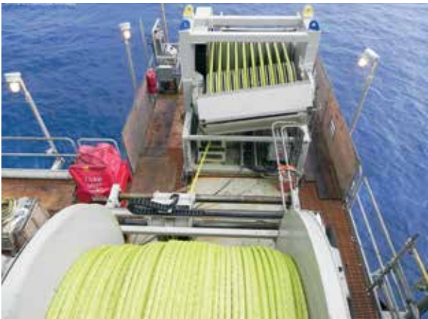
Logan's winch design includes a storage reel with capacity for 9,200 feet of 2-1/2" diameter Quantum-12 high-performance rope. Quantum-12's superior bend fatigue properties allowed a significantly smaller diameter traction head, reducing weight.
