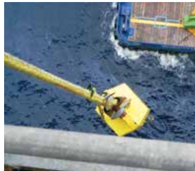
After two years of regular service, inspections show the rope to be in excellent condition with no internal abrasion.
