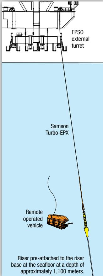
*The ROV oversees the Turbo-EPX-riser connection as the Turbo-EPX takes the full weight of the riser.*
