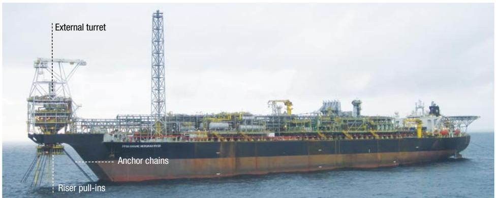
*FPSO Kwame Nkrumah is capable of processing more than 120,000 barrels of oil and producing 160 million standard cubic feet of gas per day.*
