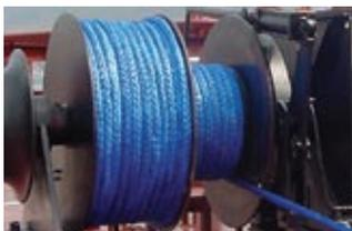
*Maintain a minimum of 8-10 wraps on the tension side of split drum winches at full extension.*
