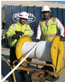
*Samson Stable Braid replaced the 3-strand nylon lines previously used to hold the ship "steady" in drydock.*
