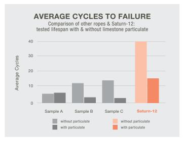
Samples impregnated with limestone particulate, tested at a relative load (10% of ABL): Saturn-12 cycles to failure were more than 5 times higher than the average of the other three ropes tested.
