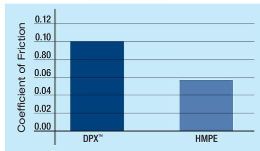
FIGURE 2 COF Comparison: DPX™ vs. HMPE
