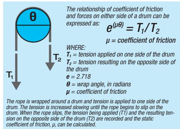
FIGURE 1 COF Measurements
