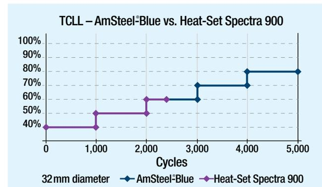
**FIGURE 1** TCLL Chart for AmSteel®Blue and Heat-Set Spectra 900.
