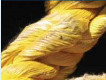
FIGURE 1 Proton-8 with a hockle.
