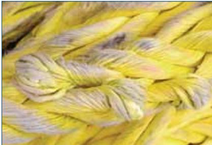
FIGURE 2 Proton-8 with severe strand hockles.
