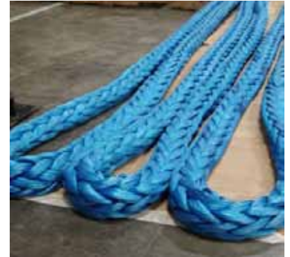
Do not allow the length of rope being measured to be curved or twisted.
