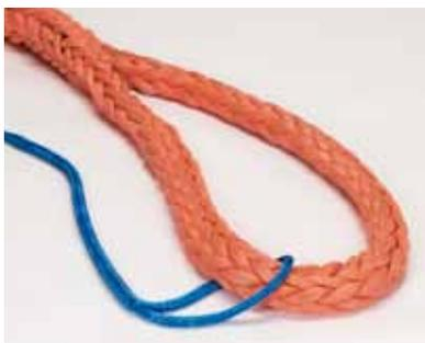
**FIGURE 4** Messenger line spliced directly to eye
