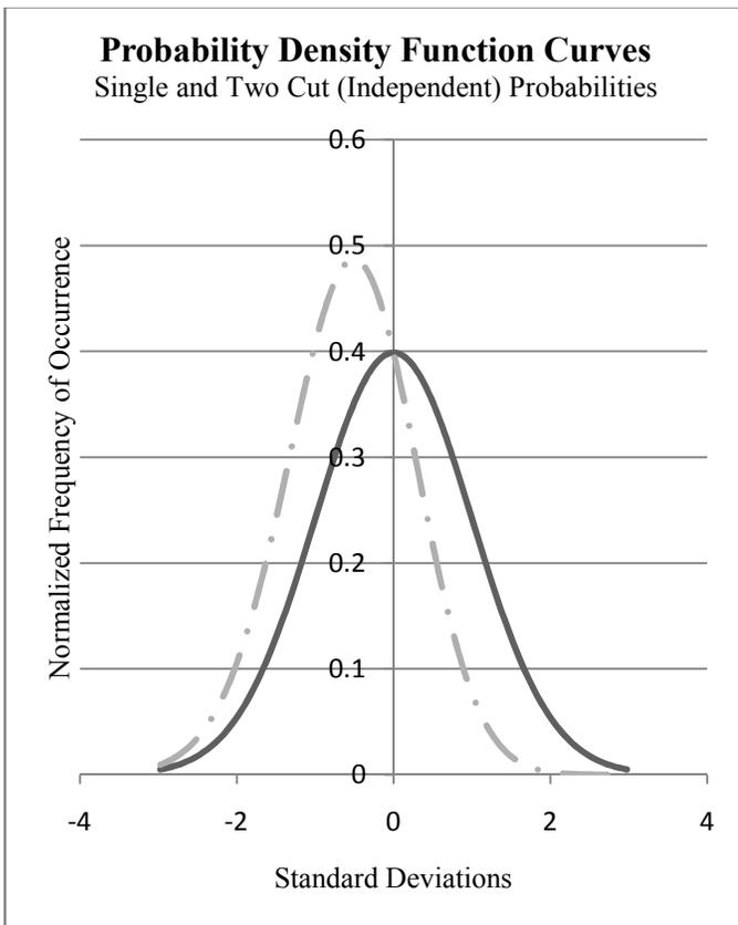
Fig. 5. Solid curve is a normalized probability density function (PDF) for a normal distribution (the average breaking strength of samples with a single cut strand is assumed to follow this distribution) while the dashed curve is the resulting PDF for the average strength of a sample with two independent weak points.
