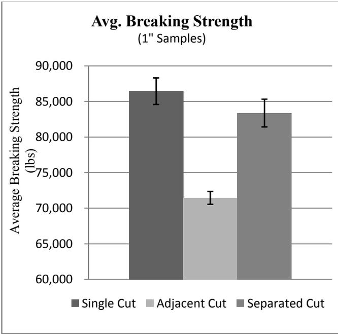
Fig. 7. Comparison of average breaking strengths for various levels of cutting damage.
