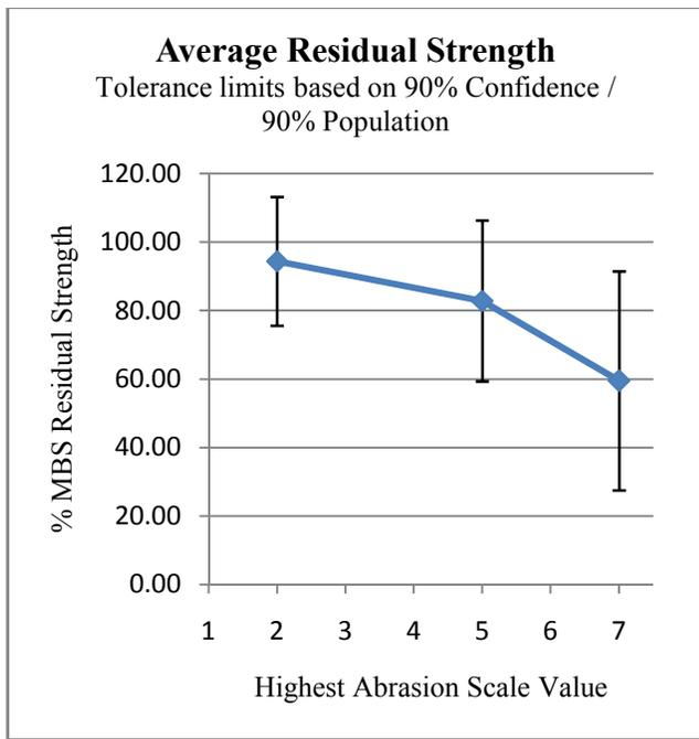
Fig. 3. Graph illustrating the average strength retention for results in each bin.
