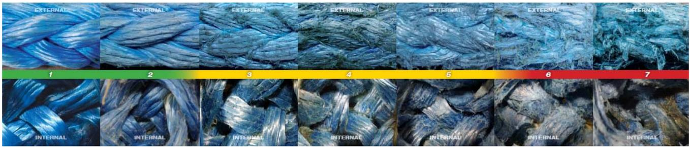
Fig. 1. Visual comparator tool illustrating the seven levels of internal and external abrasion.
