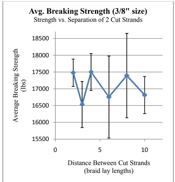
Fig. 6. Comparison of average strength based on cut separation with error bars indicating 95% confidence in the mean.
