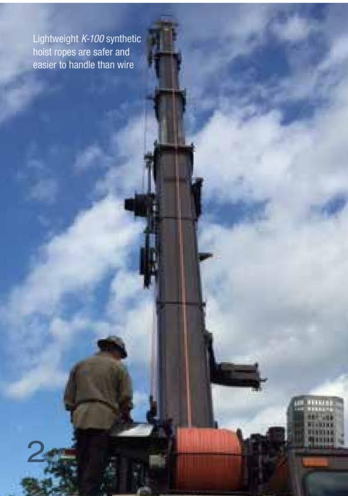
Lightweight *K-100* synthetic hoist ropes are safer and easier to handle than wire
