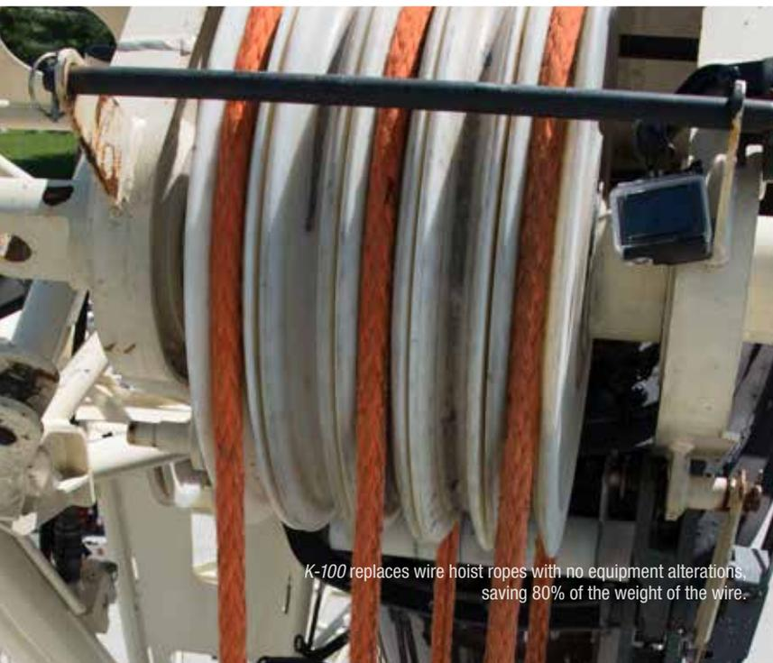
*K-100 replaces wire hoist ropes with no equipment alterations,
