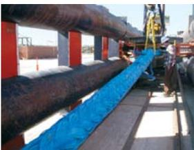
Samson manufactured the 152 mm diameter AmSteel<sup>®</sup>Blue and conducted break tests to confirm strengths. The minimum break strength for 152 mm AmSteel<sup>®</sup>Blue is 1,457 metric tons.
