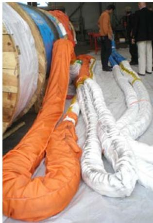
Endenburg BV fabricated the 2 sets of the slings and grommets for the project. Chafe protection was applied to all weight-bearing points.
