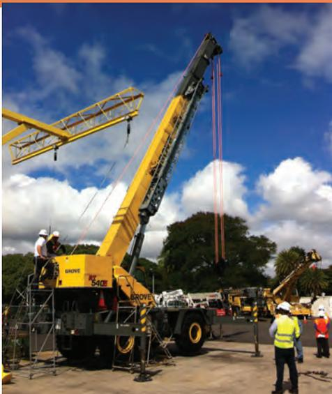
K-100 is currently installed as the main and auxiliary lines on the Manitowoc RT540E crane at Naval Station Pearl Harbor, and is also used on the Manitowoc RT9130E crane at Newport News Shipbuilding. At the Pearl Harbor location, the lines service two, eight-hour shifts per day, five days a week, loading cargo and supplies onto Navy ships.
