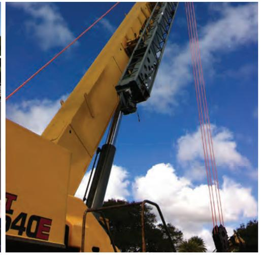
One unexpected perk surprised Navy Crane Center. During the late shift when the light is dim, workers said they liked the visibility of K-100 much better; the orange color was easier to spot and grab compared to the dull, flat tones of wire.
