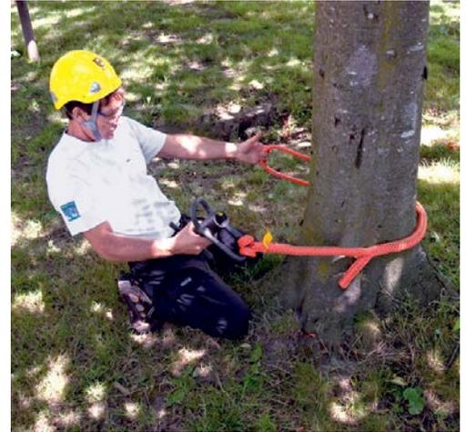
Adjustable lifting slings allow snug lifting control and minimize the number of fixed length slings required.
