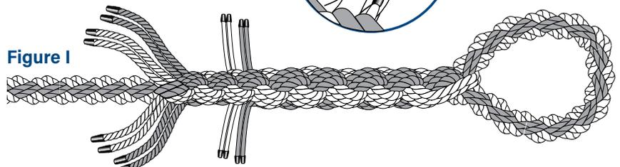
**8E** The tapering process continues by reducing the volume of the remaining strands by 1/2 (removing 1 of the 2 remaining strands.) Continue tucking the remaining strands for 3 more full tucks. Tape the remaining strands 8-10 inches from where they protrude from the rope body and cut off the remainder. The finished splice should look like Fig. J.
