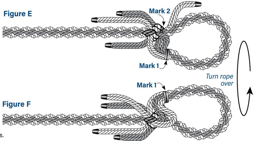
**7D** Turn the eye over and tuck the remaining (white) pair of strands under the remaining (gray) pair of strands in the standing part of the rope (Fig. F).
