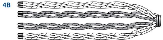
**4C** When unlaid, the strands in a pair will be twisted around each other. Untwist each strand pair so the 2 strands lie parallel to each other rather than twisting around each other. Tape the ends of each pair together.
