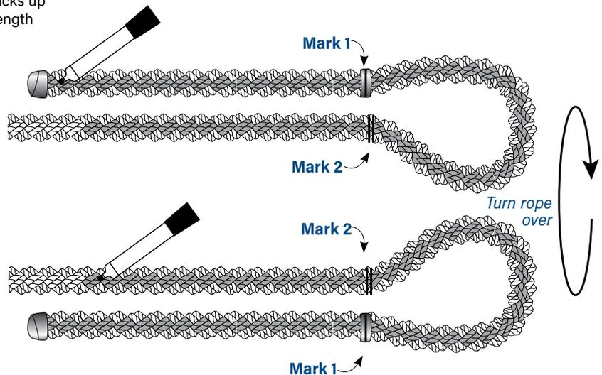
**Note:** The strands that rotate left (gray) can be marked for improved visual reference. 8-strand ropes are composed of 4 pairs of 2 strands each. 2 of the strand pairs rotate to the left, and 2 pairs rotate to the right. When marking the left-rotating strands, be sure to turn the rope over and mark the left-rotating strands on the opposite side of the braid.
