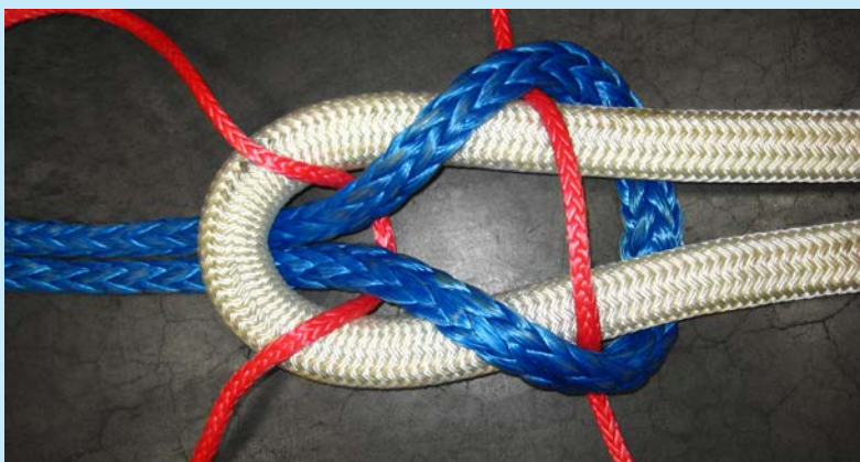
Figure 5.22: Cow hitch connection with pigtail included.
