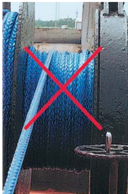
Line installed incorrectly on working side of winch drum! On working side of winch, only wrap a single layer of line (8 wraps). Working part of line should come off end of wraps, not from the middle as shown.
