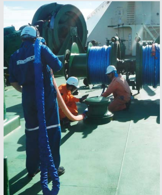
The crew performing an inspection with a slack line. Inspect the full path of the mooring lines from winch drum to chock. All contact surfaces should be free of rust, pits, or scores.
