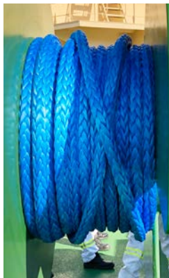
Line installed on storage side of winch drum. Crossovers prevent AmSteel®-Blue from diving between layers and getting stuck during deployment.
