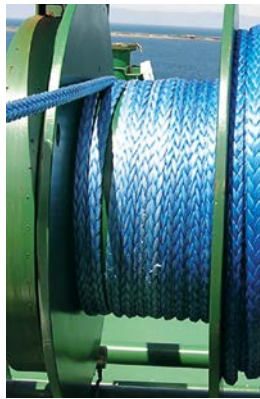
Line installed correctly on working side of winch drum. Single layer of wraps on working side of drum. Working part of line comes off one side of wraps as shown.
