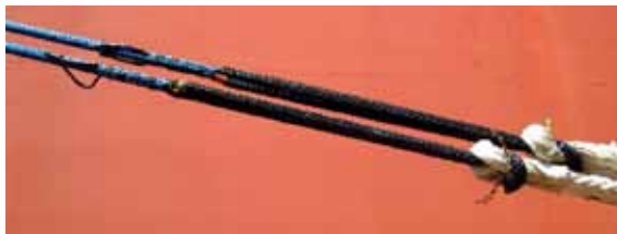
Using a braided pendant with a braided mainline will reduce the likelihood of twisting the mainline.
