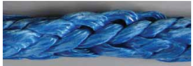
FIGURE 1 The loose strands at the top of the rope do not contribute to the strength of the rope. The tight strands at the bottom of the picture bear most of the load.
