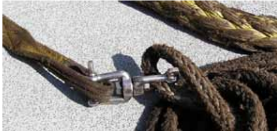
Using a swivel to connect the messenger line to the mainline or pendant can reduce twist in the pendant and mainline.
