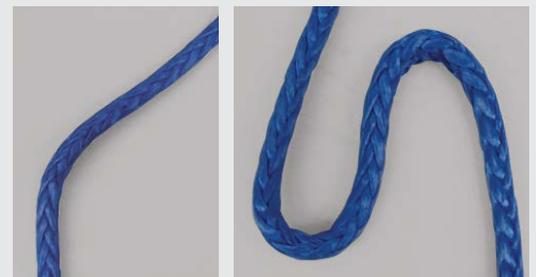
**FIGURE 3** Frozen rope bent at 45° on the left and 180° on the right
