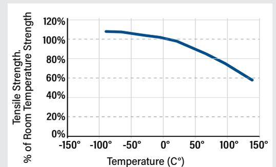
**FIGURE 2** Strength of Dyneema® fiber vs. Temperature
