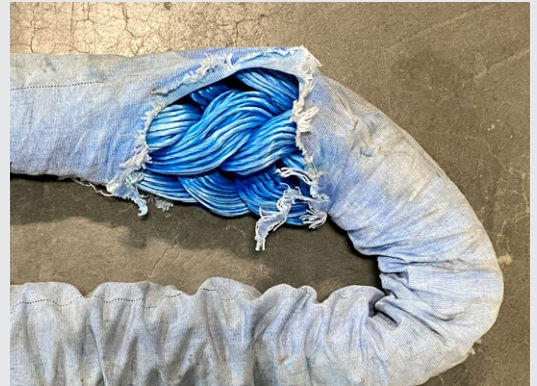
CHAFE DAMAGE = REPAIR
