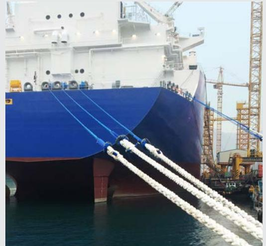
*Creep would be a factor in permanent applications such as mooring for long periods of time or guy-wire installation such as for antenna towers*
